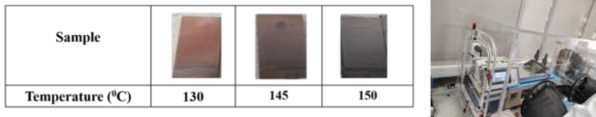
Figure 15. a) Example of FA_{0.7}K_{0.1}MA_{0.2}PbI_{2.6}Cl_{0.4} (FAMA@10K) thin films deposited by dr. Blade at different substrate temperatures; b) Slot die printing system installed in in-house made glovebox
