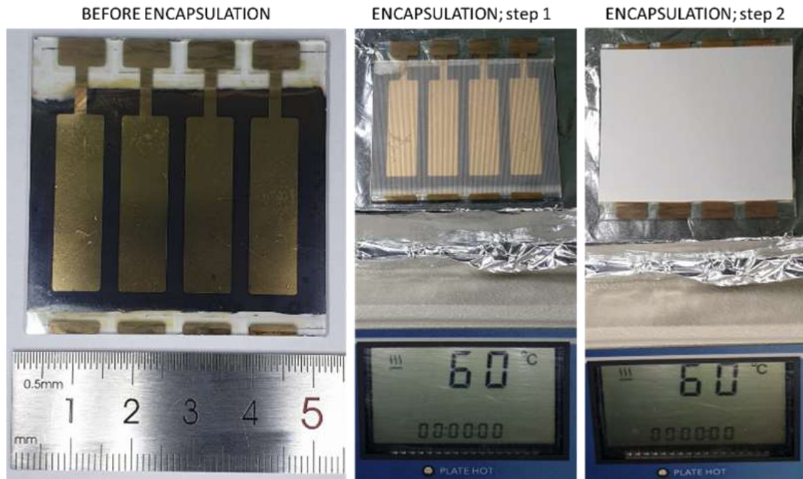
Figure 3: Encapsulation process of photovoltaic modules (5cmx5cm) of PSCs.
