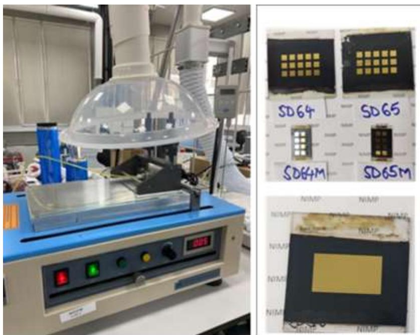
*Figure 1. Slot-die MTT machine with mobile vapor extraction used for fabricating small and large area PSCs (from  $0.083 \text{ cm}^2$  to  $4.5 \text{ cm}^2$  active areas).*
